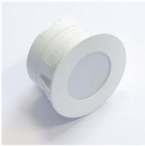
Auro is a miniature KNX motion detector, which connects directly to the bus without additional interface. Auro is the most compact full KNX motion detector on the market, with a diameter of 52mm. The inside fitting diameter is 43mm, with an installation depth of only 39mm.
